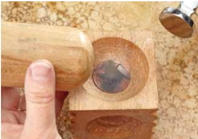
3 Using a wooden dapping block, dap the disc for a gentle curve.
