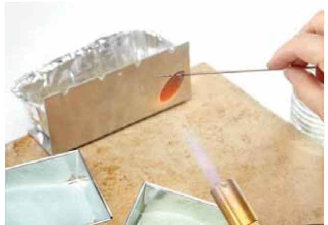
4 Place the disc on the mandrel (with the concave side facing out or away from your hand). In this case the mandrel should be as close in size to the size of the hole in the disc as possible. Enamel the disc in two to three layers of Robin's Egg. You may want to pull the bead a little closer to the end of the mandrel.
