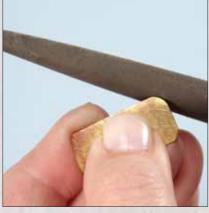
Filing Rough Edges OUse a metal file to eliminate any rough edges from the ribbon tab.
