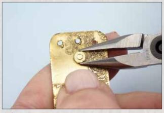
**5**Screw Bars Together Screw the two bars together with small screws and nuts. Tighten the nuts and trim excess screw stems so they are flush with the nuts. Sand the cut stems and tighten the nuts again.
