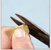
Creating Ribbon Tab Ocut the etched metal to create a tab that is  $\frac{1}{2}$ " ×  $\frac{5}{8}$ " wide. Round the corners of the tab with metal sheers.
