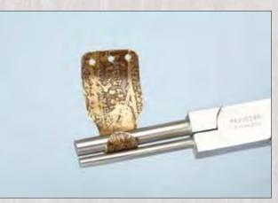
**9**Creating Hook Create a bend in the metal of the other end of the clasp. Use forming pliers to create the bend about 1/2" from end of the metal.
